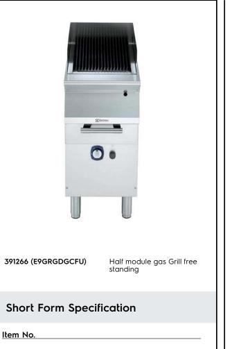
To be used with natural or LPG gas. High efficiency 11 kW stainless steel burners with self stabilizing flame. Cooking surface grids in enameled cast iron, easily removable for cleaning. Includes drip tray for the collection of grease and fat. Exterior panels of unit in stainless steel with Scotch Brite finish. Extra strength work top in heavy duty 2 mm stainless steel. Rght-angled side edges to allow flush-fitting junction between units.
